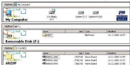
On PC, to remove the Ares-P II from the USB connection, double click first the "Unplug or Eject Hardware" icon and stop the corresponding drive letter before removing the USB cable.
